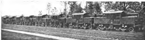
Eight of the thirty-five 100-ton 2,200 horse-power electric locomotives built for the New York Terminal electrification of the New York Central Lines by the General Electric Company and the American Locomotive Company at Schenectady, N. Y.
